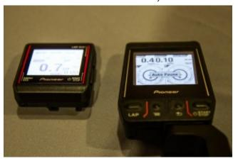
The lightweight display utilizes a 1.87-inch black and white LCD touch screen to provide a window of data including Pioneer's exclusive left and right force vector information. The robust computer can access and display left and right power output, pedaling stroke efficiency, power loss, force vector analysis, torque, cadence, heart rate, GPS positioning, speed, distance, elevation gain/loss, barometric pressure, ambient temperature, and more.
